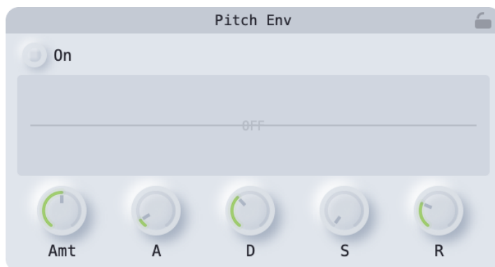
The Pitch Env panel. The display reads OFF until the envelope is switched on; it then draws the shape and is not draggable.
