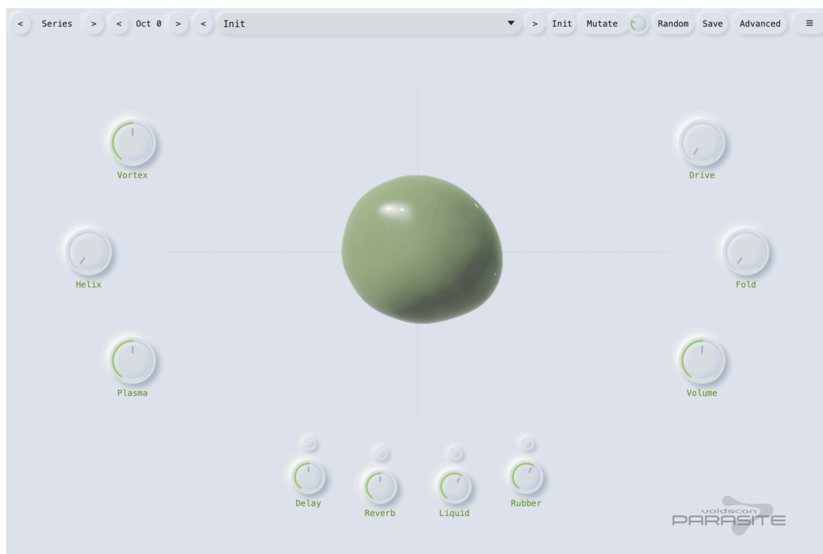
The Main page on the Init preset. The preset row runs along the top; Vortex, Helix and Plasma sit on the left, Drive, Fold and Volume on the right, and the four effects along the bottom.
