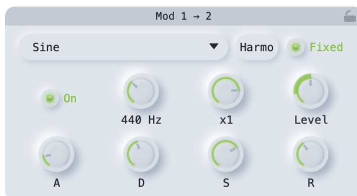
Mod 1 with Fixed pressed. The ratio knob has become a frequency in hertz and Fine has become Multi, a multiplier in steps of ten.
