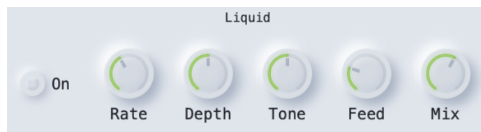
The Liquid panel. Rate reads a percentage even though it is a speed; Feed is resonance and feedback in one knob.
